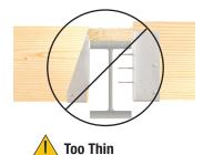
Top flange nailing cannot fully penetrate nailer, causing reduced allowable loads. Never use hangers which require multiple face nails since the allowable loads are dependent on all nail holes being used.
