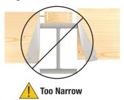
Top flange not fully supported can cause nail breakout. Or, by fully supporting top flange, hanger is tilted back, causing lifting of carried member which results in uneven surfaces and squeaky floors.
