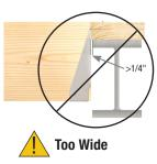
Loading can cause cross grain breaking of nailer. The recommended nailer overhang is 1/4" maximum per side.
