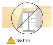
Top flange nailing cannot fully penetrate nailer, causing reduced allowable loads. Never use hangers which require multiple face nails since the allowable loads are dependent on all nail holes being used.
