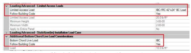
Building Code Settings in Structure with Truss Design
