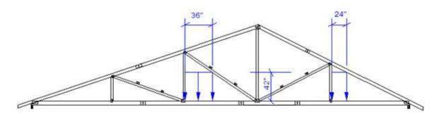
This applies to areas that are accessible via a pull-down stairway or framed opening with a bottom chord pitch of less than 2/12, or an opening of 20 inches by 30 inches where there is at least 30 inches of clearance above the opening.
