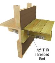
Typical DTB-TZ deck to ledger installation
