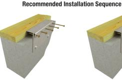
1) Install 5 - WS6 structural wood screws
