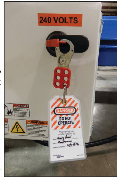
Figure 1-1: An Example of a Lockout/Tagout Device
