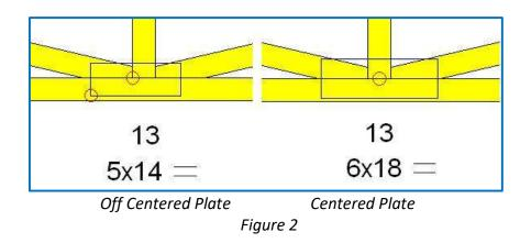
Figure 2 shows the difference in the way the program would plate a joint. Note that the off centered plate is offset in both the x and y dimensions.
