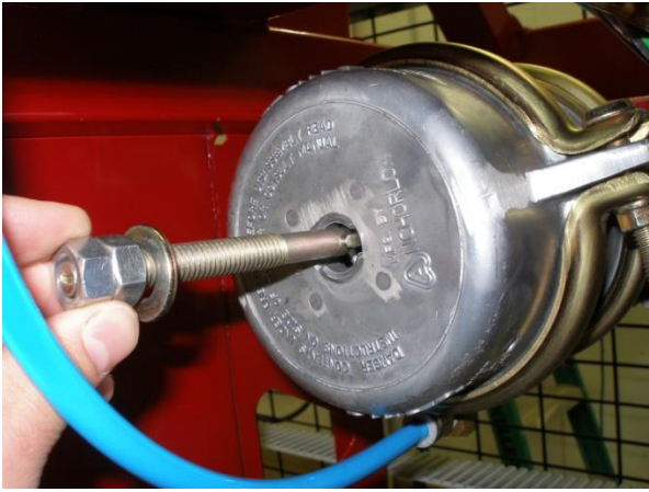
Inserting tool into the hole; aligning tabs with slots
