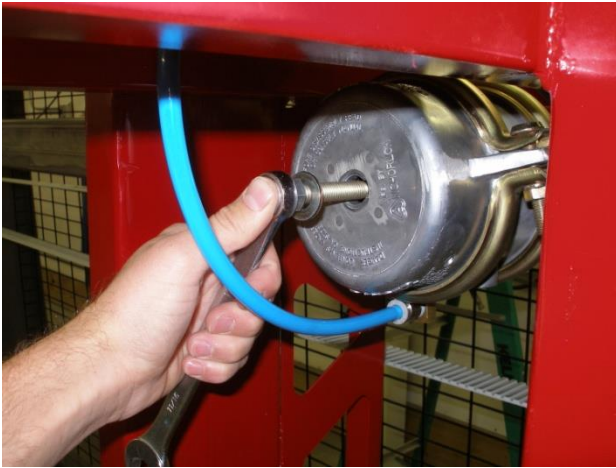
Turning release tool clockwise
