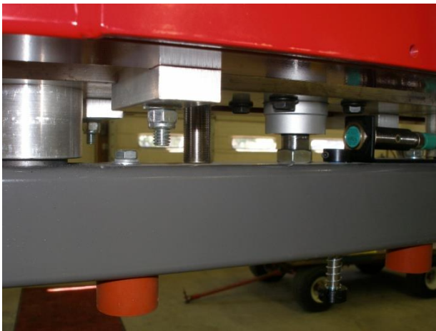
Installing Picking Head Cylinder
