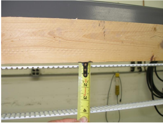
Drive Belt Tensioning – 1/4" sag
