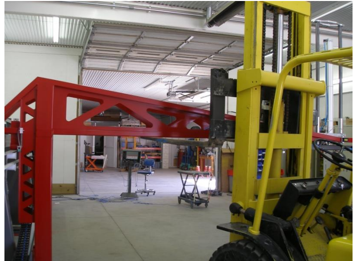
Lift Point on Gantry
