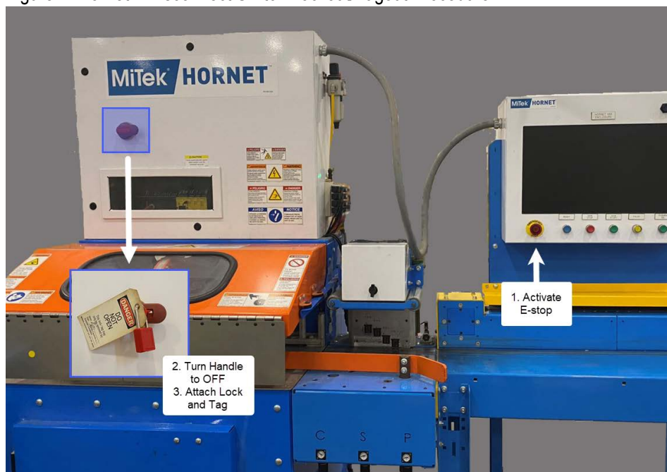
Figure 1: Hornet II Disconnect Switch Lockout/Tagout Procedure
