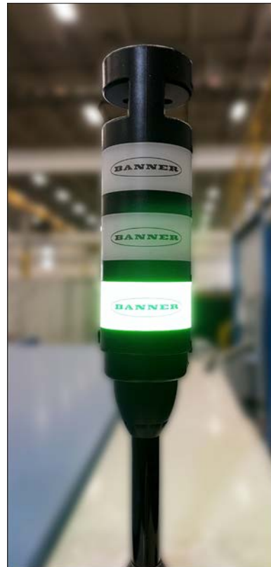
Figure 6-6: Light and Horn Beacon on Main Enclosure
