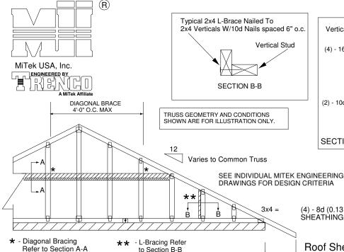
PROVIDE 2x4 BLOCKING BETWEEN THE FIRST TWO TRUSSES AS NOTED. TOENAIL BLOCKING TO TRUSSES WITH (2) - 10d NAILS AT EACH END. ATTACH DIAGONAL BRACE TO BLOCKING WITH (5) - 10d NAILS.
