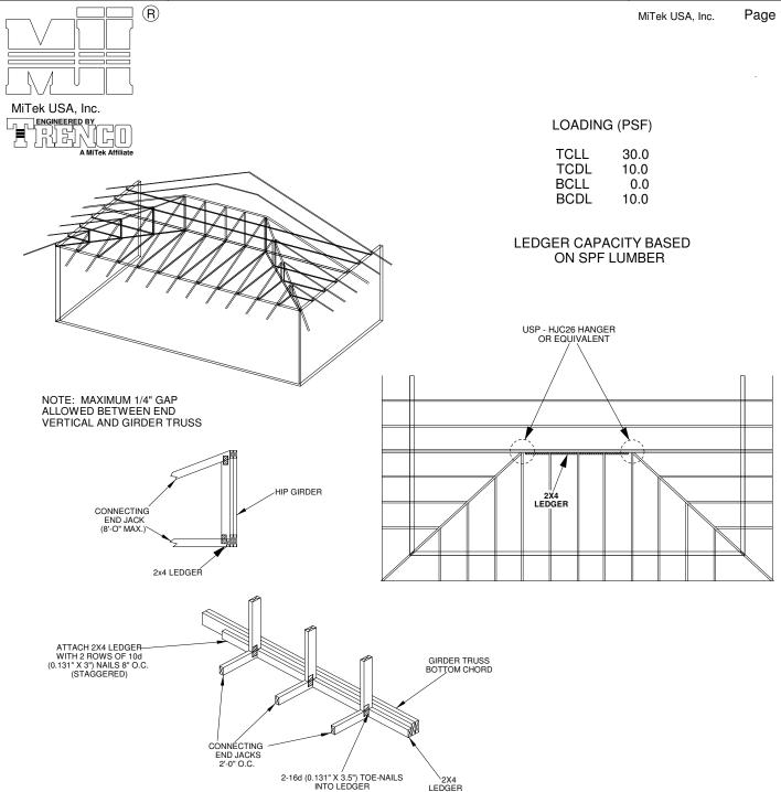
MAX MEAN ROOF HEIGHT = 30 FEET **CATEGORY II BUILDING EXPOSURE B or C** ASCE 7-98, ASCE 7-02, ASCE 7-05 120 MPH ASCE 7-10, ASCE 7-16 150 MPH WIND DURATION OF LOAD INCREASE: 1.60 MAX TRUSS SPACING = 24" O.C. MAX STUD SPACING = 24" O.C. MINIMUM PITCH 3/12 MAXIMUM PITCH 12/12
