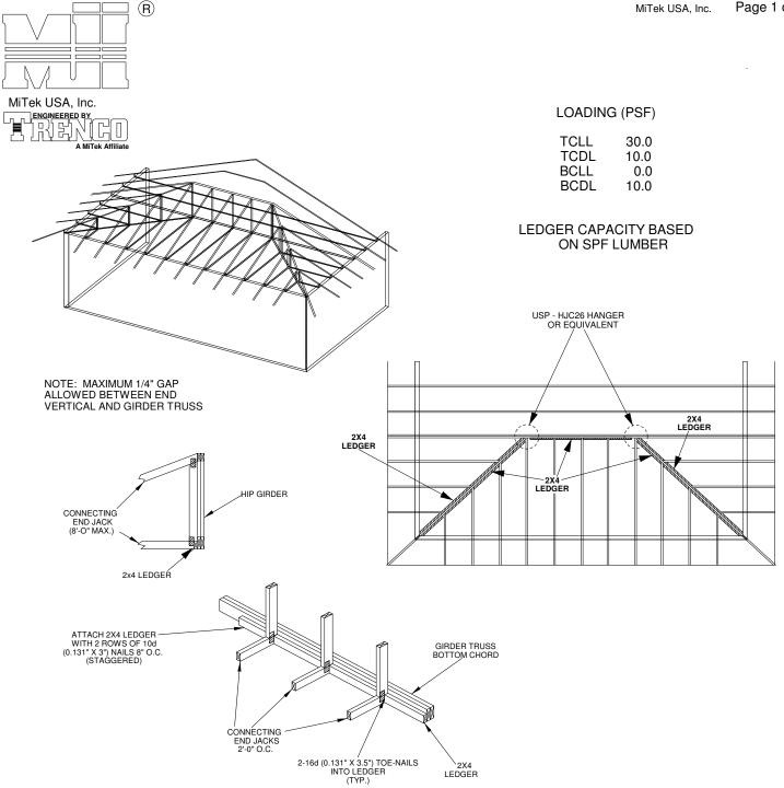
MAX MEAN ROOF HEIGHT = 30 FEET CATEGORY II BUILDING **EXPOSURE B or C** ASCE 7-98, ASCE 7-02, ASCE 7-05 120 MPH (MWFRS) ASCE 7-10 150 MPH (MWFRS) WIND DURATION OF LOAD INCREASE: 1.60 MAX TRUSS SPACING = 24" O.C. MAX STUD SPACING = 24" O.C. MINIMUM PITCH 3/12 MAXIMUM PITCH 12/12
