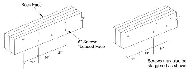
It is vitally important that the plies are tightly clamped together during the installation of the screws to prevent gaps between the plies.
