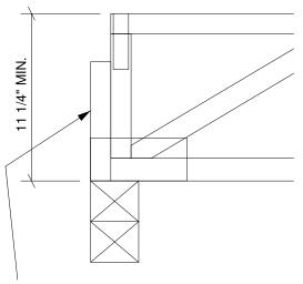
FASTEN RIBBON BLOCK TO END VERTICAL WITH TWO ROWS OF 10d (0.120" X 3") NAILS SPACED 4" O.C. (USE THREE NAILS MINIMUM)
