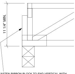
FASTEN RIBBON BLOCK TO END VERTICAL WITH TWO ROWS OF 10d (0.120" X 3") NAILS SPACED 4" O.C. (USE THREE NAILS MINIMUM)
