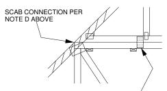
FOR ALL WIND SPEEDS, ATTACH MITEK NP37 20 GA Nail-On PLATES TO EACH FACE OF TRUSSES AT 48" O.C. W/ (4) (0.131" X 1.5") PER MEMBER. STAGGER NAILS FROM OPPOSING FACES ENSURE 0.5" NAIL EDGE DISTANCE
