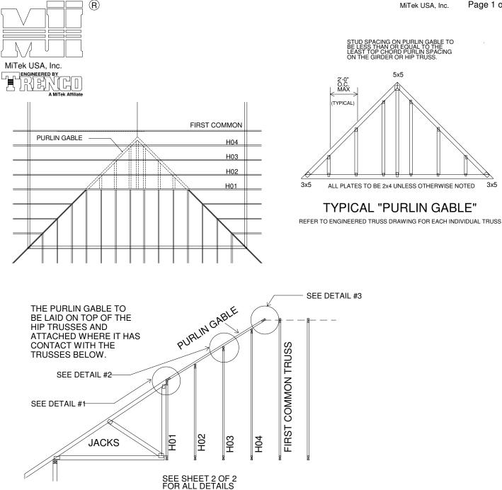
MAX MEAN ROOF HEIGHT = 30 FEET CATEGORY II BUILDING EXPOSURE B or C ASCE 7-98, ASCE 7-02, ASCE 7-05 130 MPH (MWFRS) ASCE 7-10, ASCE 7-16 160 MPH (MWFRS) WIND DURATION OF LOAD INCREASE : 1.33 MAX TRUSS SPACING = 24" O.C. MAX STUD SPACING = 24" O.C. MINIMUM PITCH 2/12 MAXIMUM PITCH 12/12
