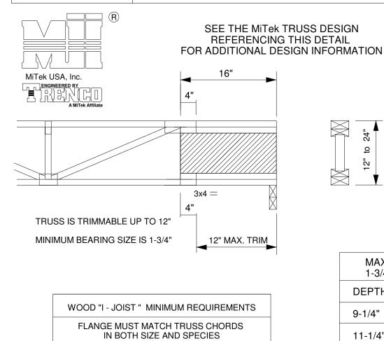
REACTION LIMITS WITHOUT WEB STIFFENER MUST BE = TO OR > THAN REACTIONS SHOWN
