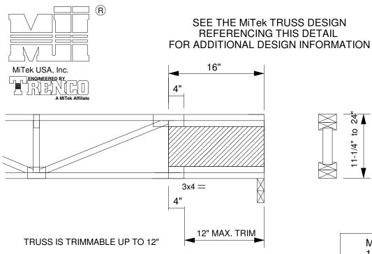
8-1/4" to 21" TRIM FIT I-BLOCK PLATED IN PLANE OF TRUSS
