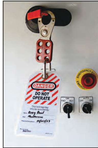
Figure SAFETY-2: Sample Lockout/tagout Device
