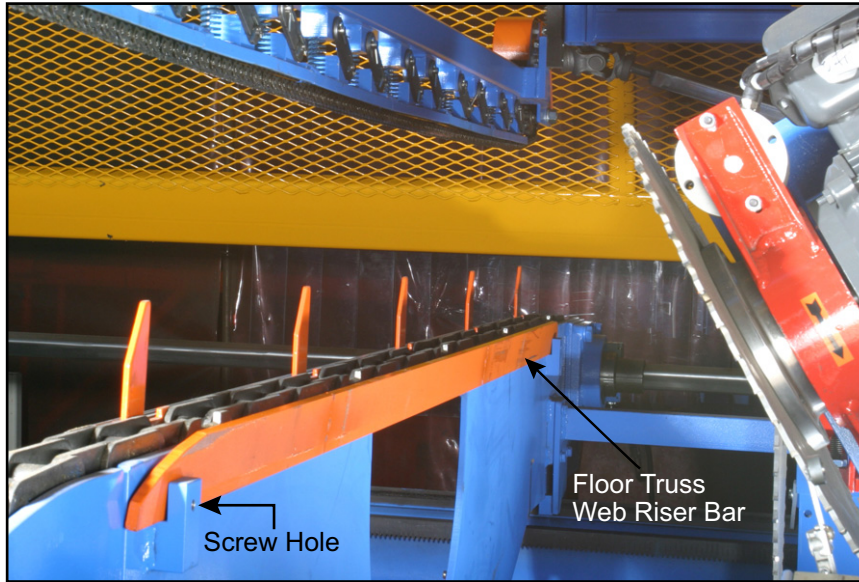
Figure 3-13: Attaching the Floor Truss Web Riser Bars
