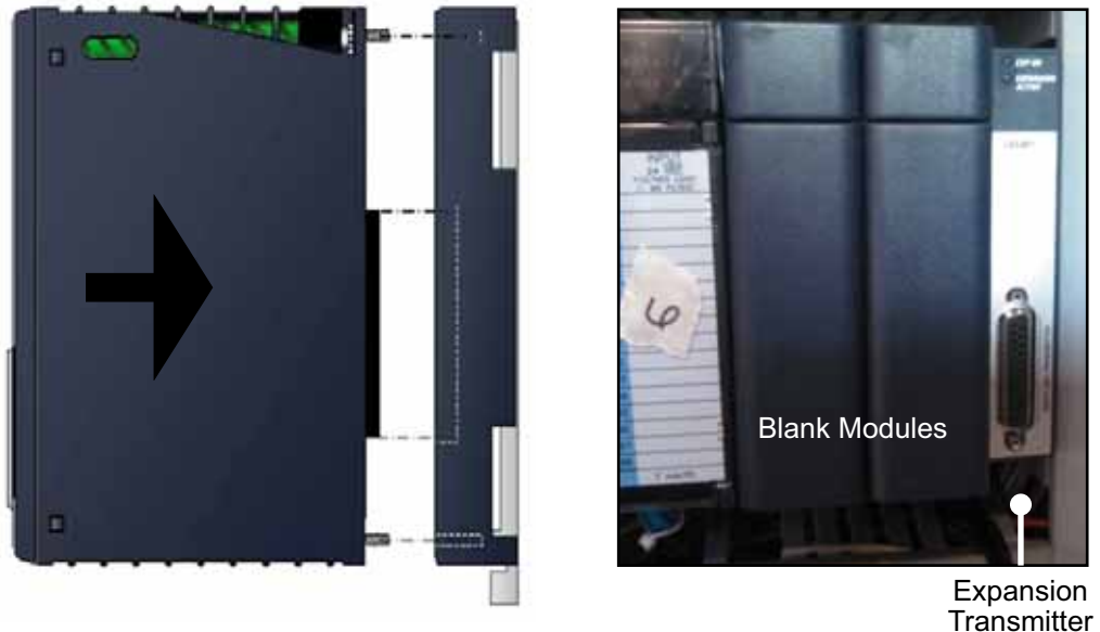
Figure 15: Installing the Expansion Transmitter Module
