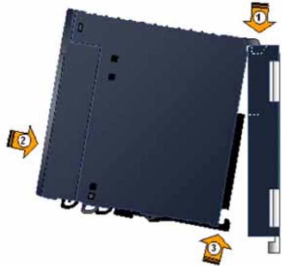
Figure 5: Installing a Pivot-Hook Module
