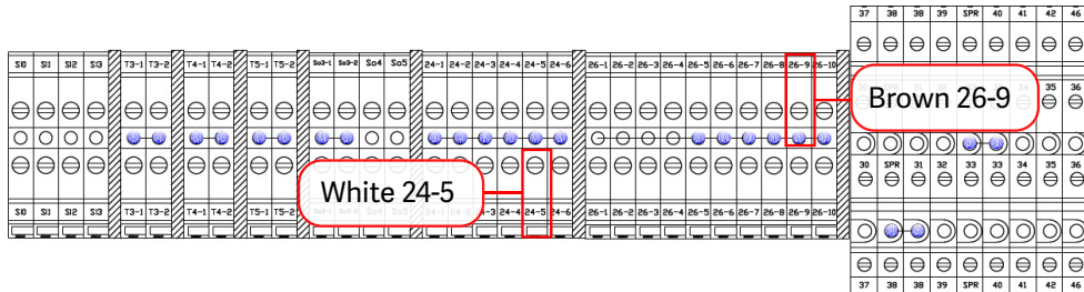
Figure 14: Existing Wires to Remove for Right Transmitter
