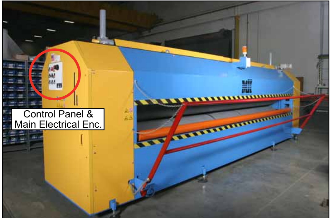
Figure 3-4: Location of Control Panel
