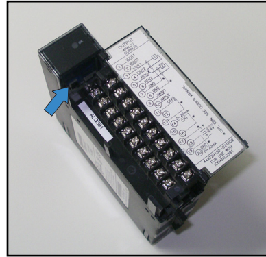
Figure 2-71: Push Lever Up to Release Terminal Strip
