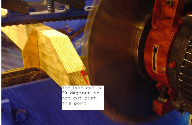
Figure B-9: Checking Pivot Point
