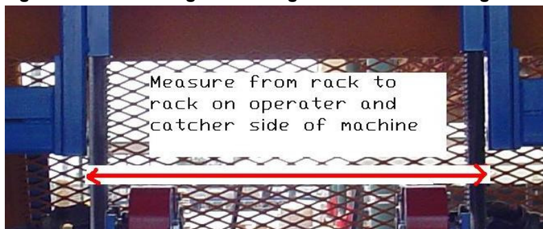
Figure B-4: Measuring the Carriage-End Hold-Down Alignment
