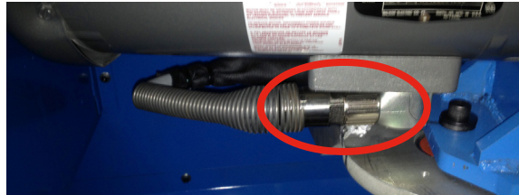
Figure 7: Connection Point at Saw Blade Motor
