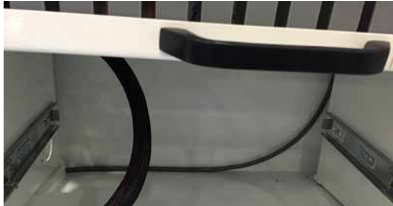
Figure 9: End-to-End Cable at Back of Enclosure
