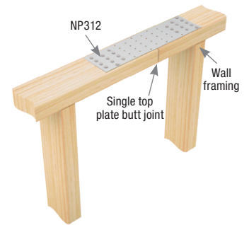
Typical NP312 prescriptive top plate splice installation
