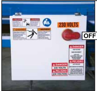
Auto Deck Enclosure May be replaced with optional infeed equipment. Power can also be disconnected using saw's main disconnect switch.
