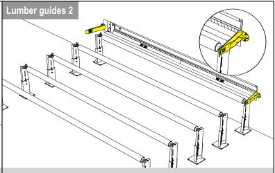
You may also mount lumber guides to the interior of a wall on the infeed side of the press. Note that infeed pull-cords are not shown here for clarity.
