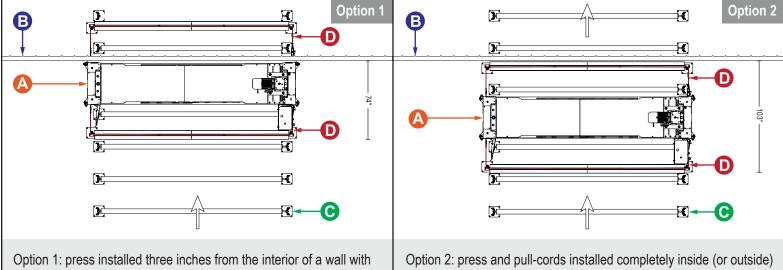
Option 1: press installed three inches from the interior of a wall with outfeed pull-cord mounted to unistrut on the exterior of wall. MiTek recommends this installation. Option 2: of the faci personnel
