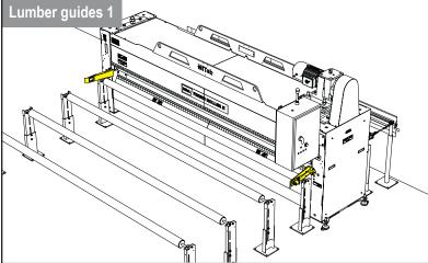
Lumber guides are mounted to the infeed side of the press. In this example, they are mounted directly to the frame. Note that infeed pull-cords are not shown here for clarity.
