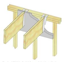
Typical FWHL Solid Sawn Joist Installation
