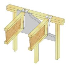
Typical FWHL I-Joist Installation
