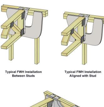
Typical FWH Minimum 2-Ply Solid Sawn Header Installation
