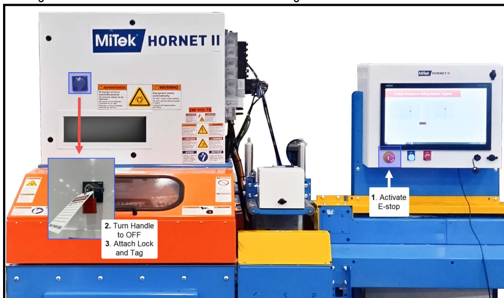
Figure 1: Hornet II Disconnect Switch Lockout/Tagout Procedure
