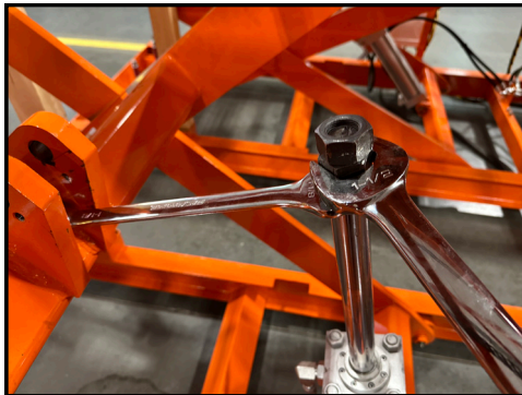
Figure 11: Loosening Cylinder Stud
