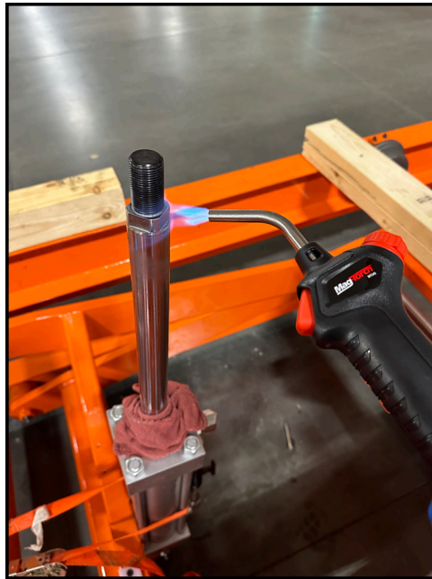
Figure 9: Heating the Cylinder Stud
