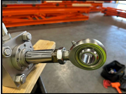
Figure 12: New Rod End Installed
