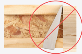
⚠️ HANGER NOT PLUMB
